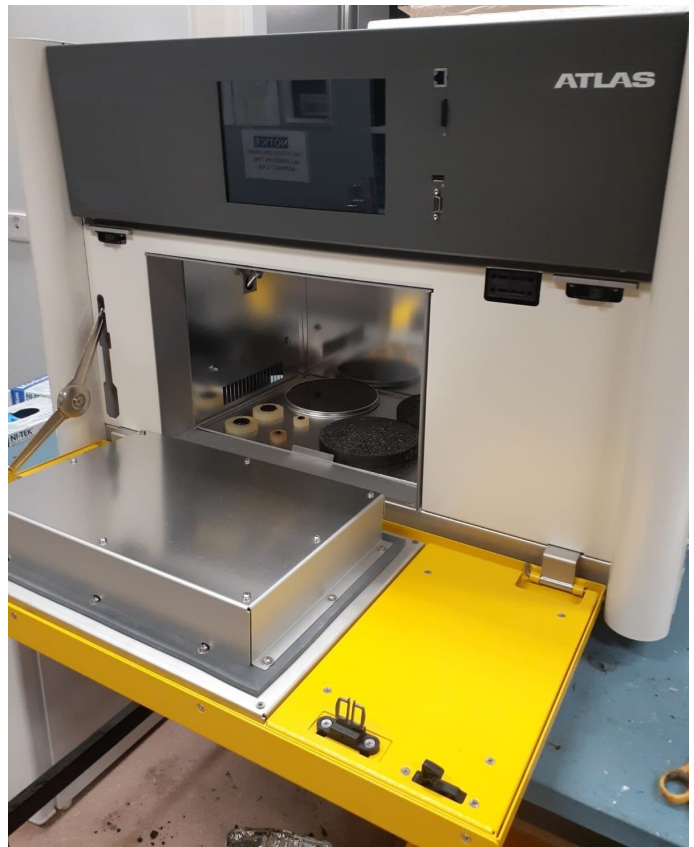
The UV machine used during testing at RMIT University. Credit: RMIT University
