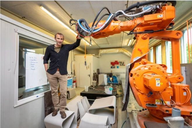
Andreas Trummer and his team have been working intensively with the institute's own concrete 3D printer for several years in the robot design laboratory. The goal: massive material savings in concrete construction. Credit: Lunghammer—TU Graz
