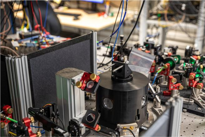
Alice, the receiver of the teleported quantum information. Inside the black aluminium cylinder, the diamond sample is cooled to  $-270^{\circ}\text{C}$ , to reduce the noise from the environment and enable the quantum control. Credit: Marieke de Lorijn for QuTech
