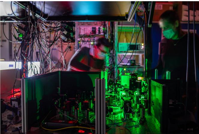
Researchers work on one of the quantum network nodes, where mirrors and filters guide the laser beams to the diamond chip. Credit: Marieke de Lorijn for QuTech.
