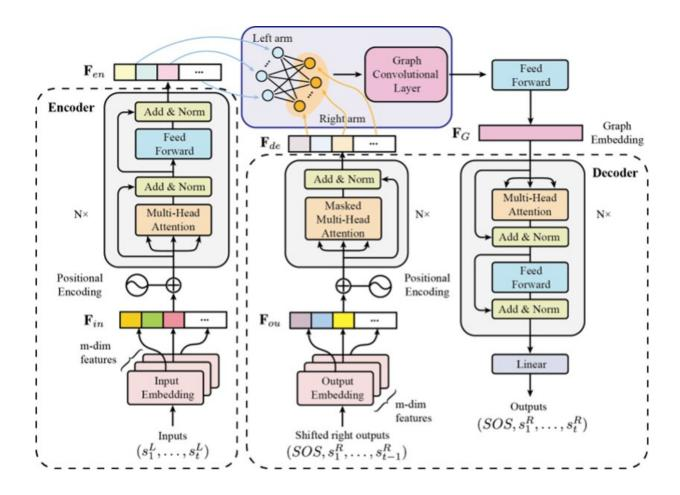
Structured-Transformer is a bimanual coordination mechanism that regards coordination as a sequence transduction problem and learns coordination by embedding a Graph Convolutional Layer halfway through the Transformer decoder to explicitly consider the robot hardware structure. Credit: Liu et al.
