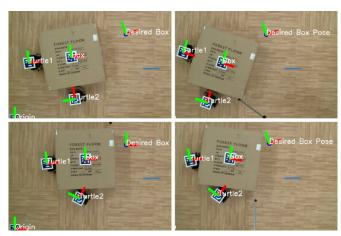
A new general-purpose optimization tool can improve the performance of many autonomous robotic systems. Shown here is a hardware demonstration in which the tool automatically optimizes the performance of two robots working together to move a heavy box. Credits: Courtesy of the researchers
