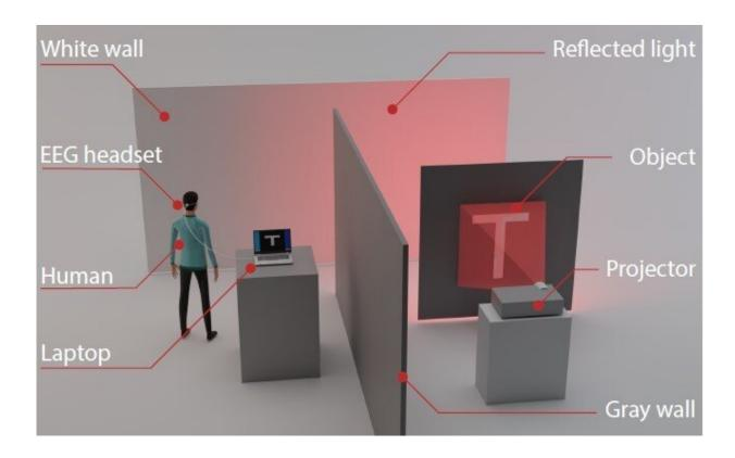
Experimental set-up for non-line-of-sight ghost imaging with EEG neurofeedback. Credit: Optica
