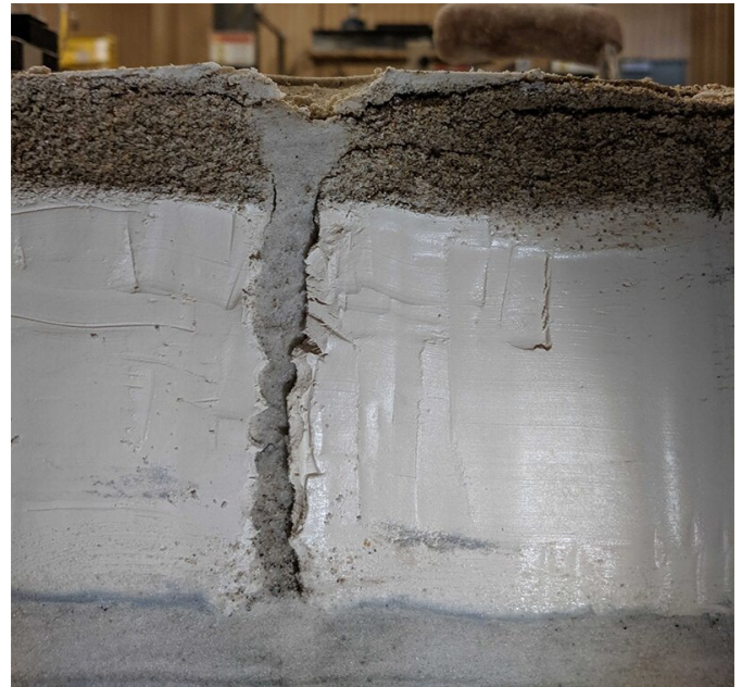
Close-up of excavated model showing evidence of sand boil due to liquefaction going through the impermeable crust. Credit: Sinha et al.
