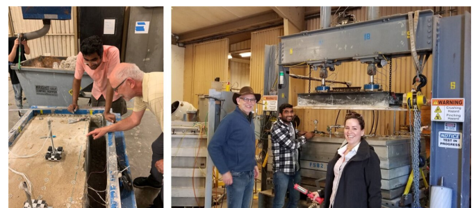
Left: Sumeet and Bruce inspecting the model (from the SKS02 test) after testing and gradually excavating. Right: Sumeet, Bruce and Katerina next to consolidation press preparing the model for SKS02. Credit: Sinha et al.
