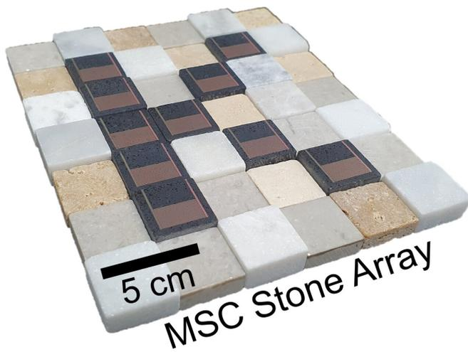
Interconnected microenergy devices built on marble tiles create customizable 3D power supply systems. Credit: *ACS Nano*
