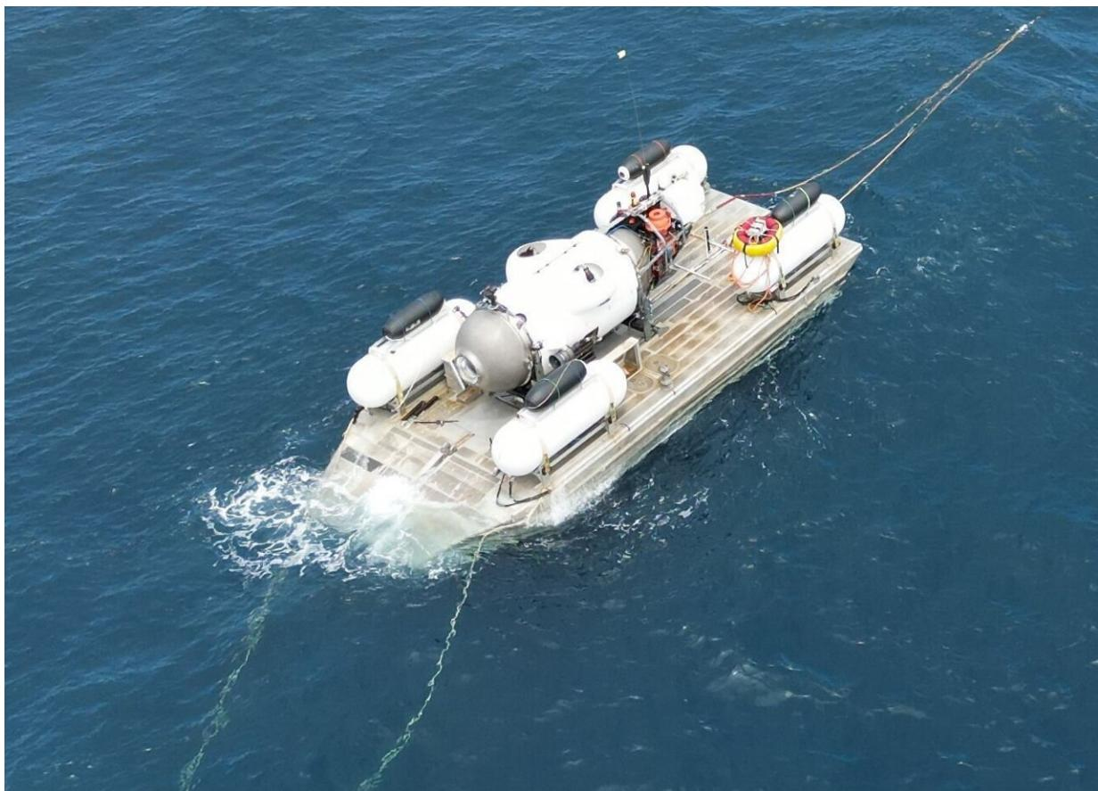
The submersible for the dive to the Titanic on its launch and recovery platform.
