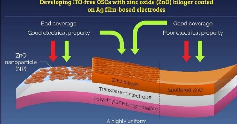
A highly uniform sputtered ZnO and blade-coated ZnO NP bilayer is used to create ITO-free electrodes
