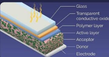
Most OSCs use indium tin oxide (ITO) as electrodes due to their high surface energy and wettability
