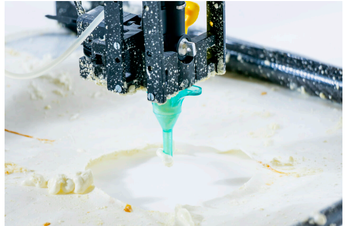
3D printing with cementitious material. Credit: University College London, Department of Computer Science, London. Dr Vijay M. Pawar & Robert Stuart-Smith, Autonomous
