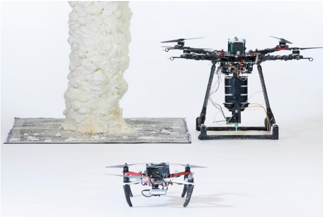
3D printing with cementitious material. Credit: University College London, Department of Computer Science, London. Dr Vijay M. Pawar & Robert Stuart-Smith, Autonomous
