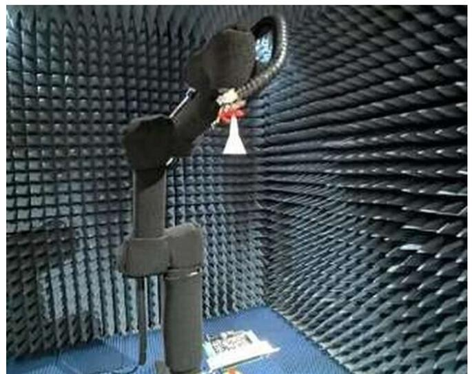
Measurement setup of the space-time-coding metasurface antenna in a microwave anechoic chamber. Credit: Wu et al.
