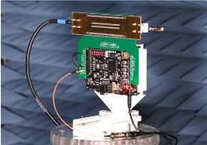
Photograph of the space-time-coding metasurface antenna. Credit: Wu et al.
